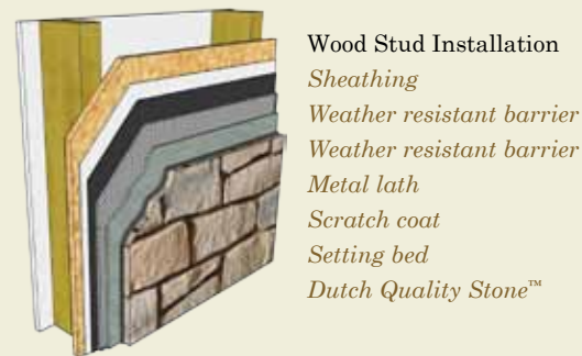
Clean Masonry Installation Scratch coat Setting bed Dutch Quality Stone™
